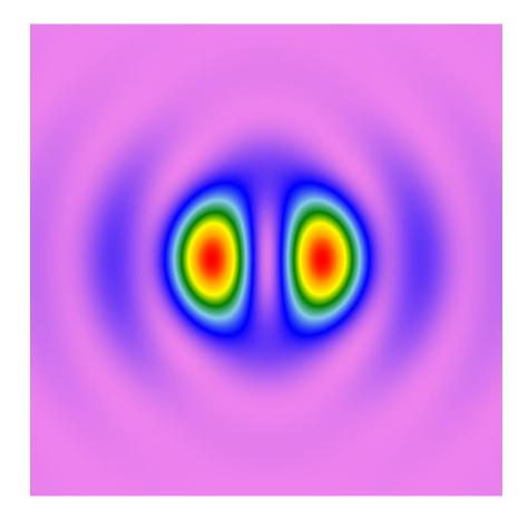
To fully characterize the focusing behavior of an ultrashort pulse, different electromagnetic properties must be considered. That includes both spatial distribution, temporal / spectral distribution, vectorial effect, and also the possible coupling amongst all the above. As an example, the focusing process of a 10fs pulse by using a high-NA parabolic mirror is modeled in VirtualLab, and both the spatial and temporal behaviors are investigated.
